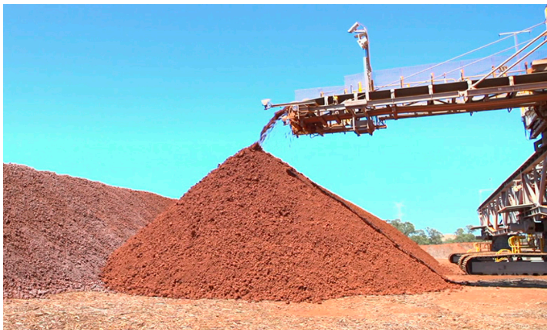
Figure 1. Example of filter press cake dry stacking with residual moisture lower than 30%
